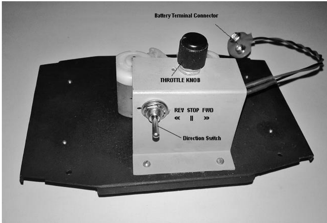
Loco Controls (above)
