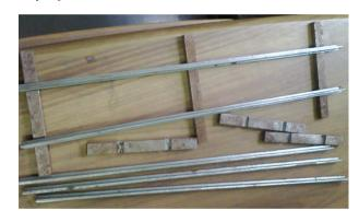
${\it Plated/un-plated Steel \ Display \ tracks \ for \ displaying \ or \ test \ running \ Locomotives \ \& \ Rolling \ Stock}$
